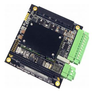
The TPSi1000-5-12 is an isolated PC/104-Plus power solution for use in embedded applications requiring isolation. The wide-range input voltages, transient suppression, isolation and pluggable terminal mating plugs make the TPSi1000-5-12 ideal for use in rugged and hostile applications. Designed tough for harsh environments including military standards, shock, vibration and extended temperature.
