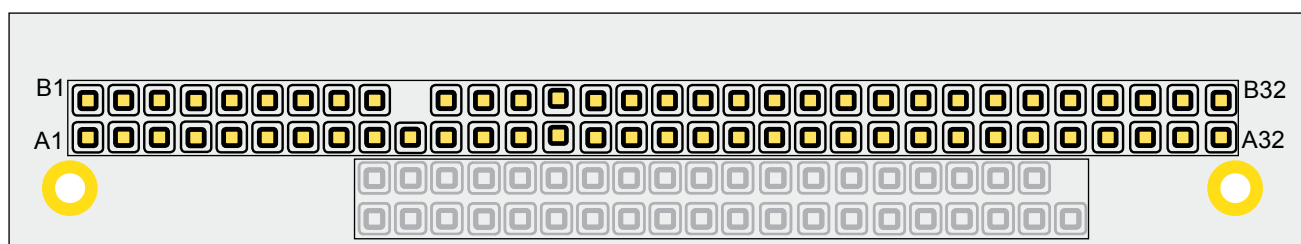
Figure 4: CN1 Connector Pinouts
