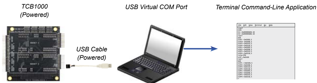
Figure 13: TCB1000 accessed using a USB cable as a Virtual COM Port
