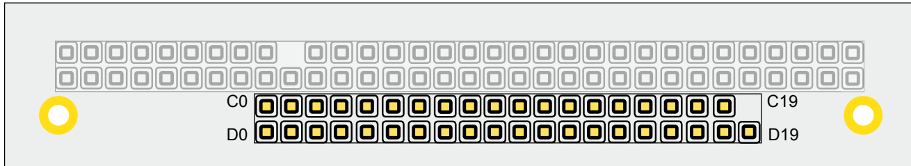
Figure 5: CN2 Connector Pinouts
