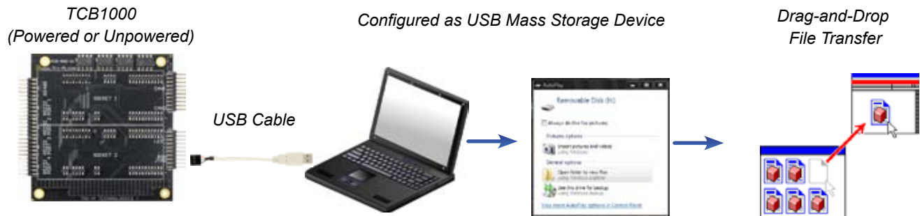
Figure 15: TCB1000 configured as a Mass Storage Device
