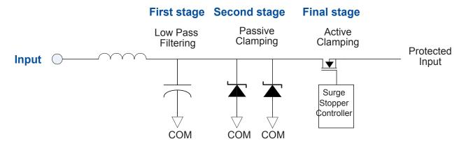
The first stage is a waveform modification that employs a low pass filter to eliminate unwanted high frequencies from entering the system.
