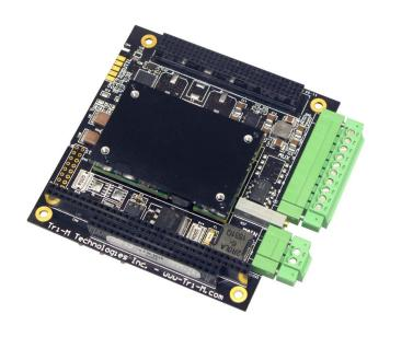
The TPSi2100 is an isolated PC/104-*Plus* power solution, designed for embedded applications requiring isolation and clean power in rugged environments.
