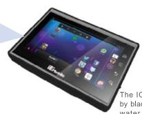
The ICECARE-05 is surrounded by black rubber protecting it from water and dust intrusions and drops.
