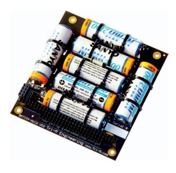
The BAT104 is a 8.4V nominal @ 2700mAh NiMh battery module that when combined with a Tri-M HESC or HPSC smart charging power solution creates a complete uninterpretable power system (UPS) in a PC/104 footprint. Designed as a rugged backup power source, the BAT104 supplies backup power and includes current and thermal fuse protection and digital temperature sensor monitoring. The BAT104 is well suited for rugged environments
