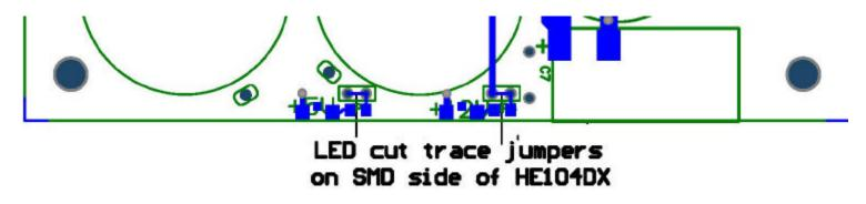
Each LED is enabled by factory default. To disable any LED, remove the LED jumper (or cut the small PCB trace if no jumper is installed) associated with the LED. To re-enable any LED, re-install the associated jumper (or solder a short jumper wire between each of the jumper pads).
