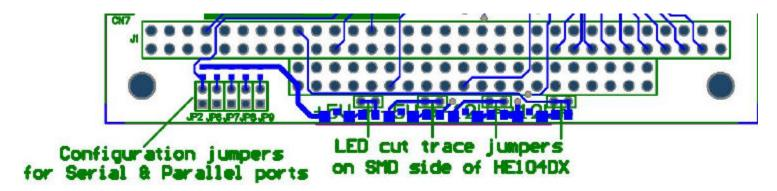
Each LED is enabled by factory default. To disable any LED, remove the LED jumper (or cut the small PCB trace if no jumper is installed) associated with the LED. To re-enable any LED, re-install the associated jumper (or solder a short jumper wire between each of the jumper pads).
