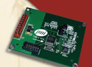
The TCM2.5 is a **drop-in replacement** for PNI's original TCM2 family of products. It offers improved accuracy and performance for compass heading, tilt and magnetometer measurements. It is the **same size**, has the **same 10-pin RS-232** interface connector and is **completely backwards compatible** with the original TCM2 ASCII protocol. These features make the TCM2.5 the choice for existing applications that require compatibility the TCM2 family of products.
