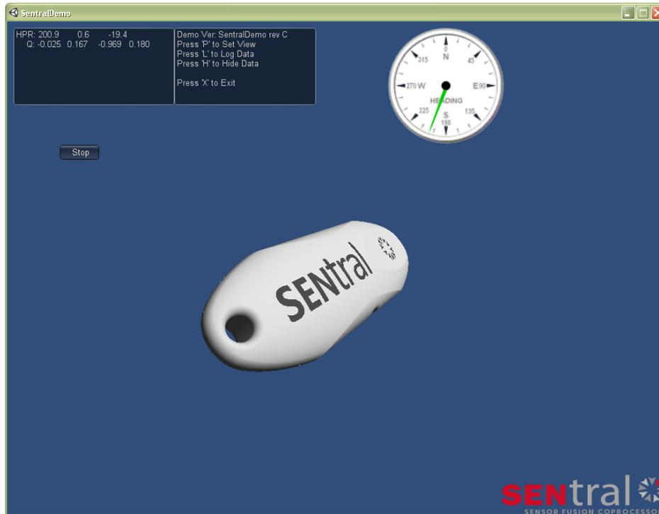
The data text box displays heading, pitch, and roll, in degrees, on the top line, and on the second line the quaternion values, Qx, Qy, Qz, and Qw.
