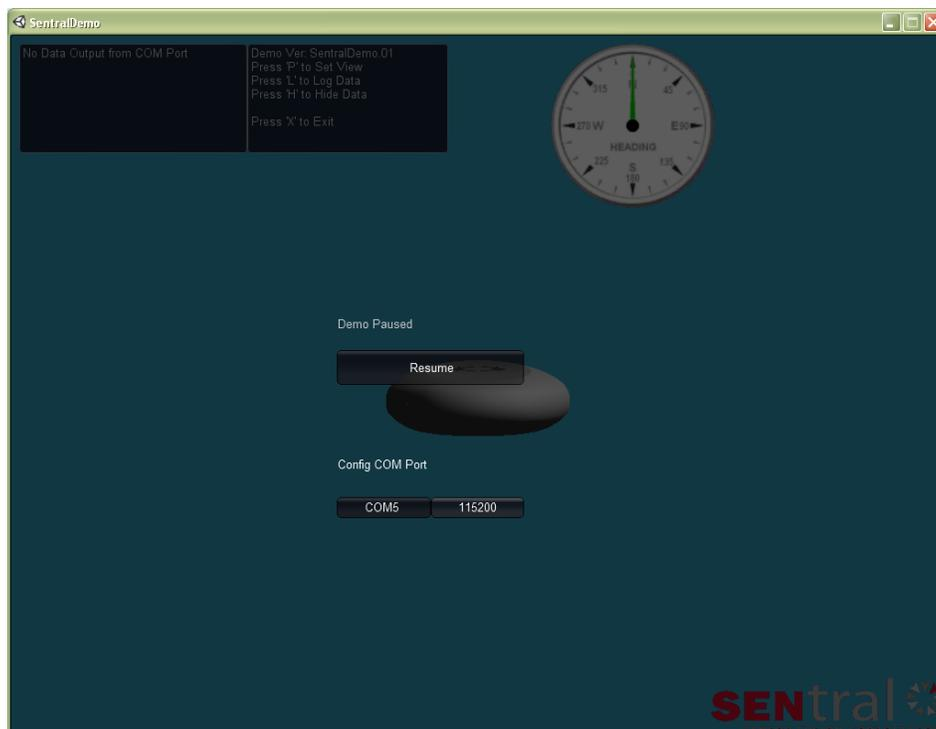
Once the program is running: 1) the whole screen will brighten, 2) the values in the upper left-most box, referred to as the data text box, are no longer “0” and will change when the module is moved, and 3) the compass dial will start tracking heading.
