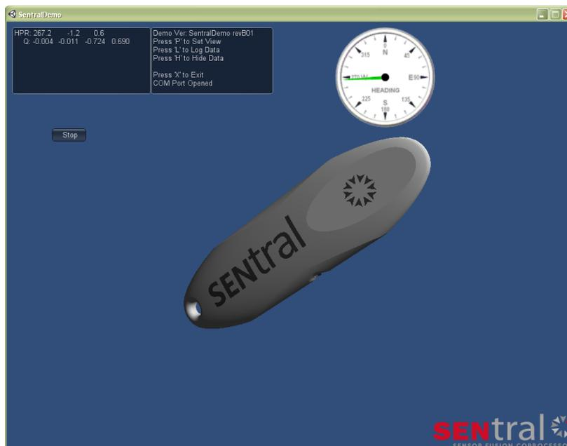
The data text box displays heading, pitch, and roll, in degrees, on the top line, and on the second line the quaternion values, Qx, Qy, Qz, and Qw. If desired, you may hide the data and command text boxes by pressing “h” on your keyboard. Pressing “h” again will toggle them back.
