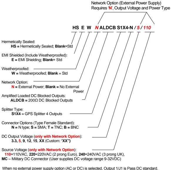
Whenever an external power supply option is selected, all outputs are DC blocked standard.
