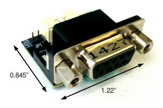
The TTL2RS232-DB9 is connected to TUP1000, TPS1000 and TPC1000 via a ten wire interconnect cable and converts the TX and RX TTL signals to RS232 levels. The TTL2RS232-DB9 also provides a micro-USB connector to plug a USB cable to a host CPU. A jumper shunt permits setting the TUP1000, TPS1000 and TPC1000 into programming mode.
