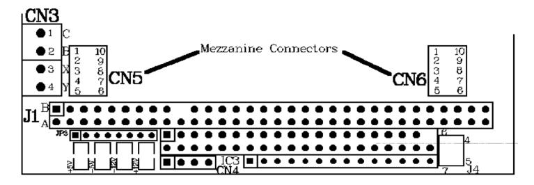
in the range of 6.5 to 20VDC through the Battery Power Connector CN3. Two external signals can be connected to the battery terminal block for use by add-on modules plugged into the mezzanine header connectors. Connect to the HE104 Battery Terminal Block as follows:
