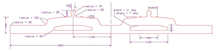
Figure 3: Cross Section of Shock Mount Pad
