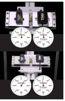
When exposed to magnetic distortion, TRAX maintains accurate heading — while the leading AHRS is thrown off track.
