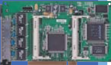
MLAN-104SSL Support 4X Gigabit LAN
