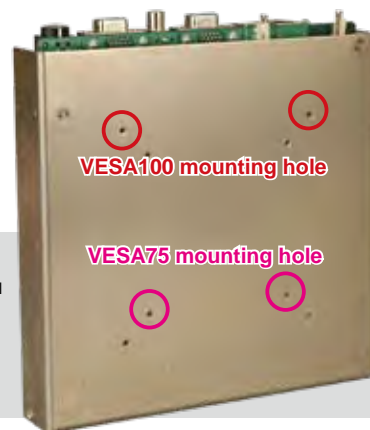
Flexibility screw mounting holes for all directional thermal solutions.
