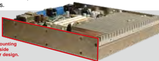
Flexibility screw mounting holes for all directional thermal solutions.
