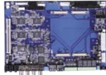
ETX-DB-DVR1 ETX Baseboard with 4 Capture Engine CF II, Dual LAN, Audio & D I/O
