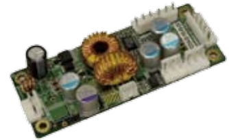
ECW-281B has two power input interfaces: 3-pin terminal block or DC power jack.
