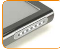
Membrane Keypad for LCD On/Off, Brightness Down/Up, Volume Down/Up, Lock, Ambient Light Sensor On/Off Control
