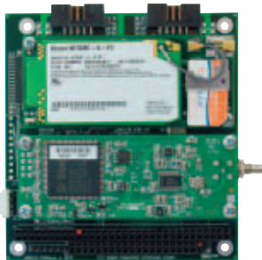
Janus-MM with GSM and GPS modules installed
