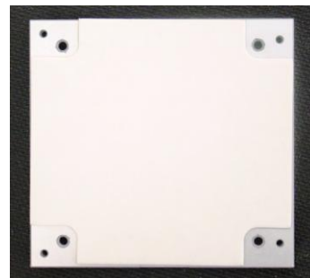
Thermal pad on heat spreader
